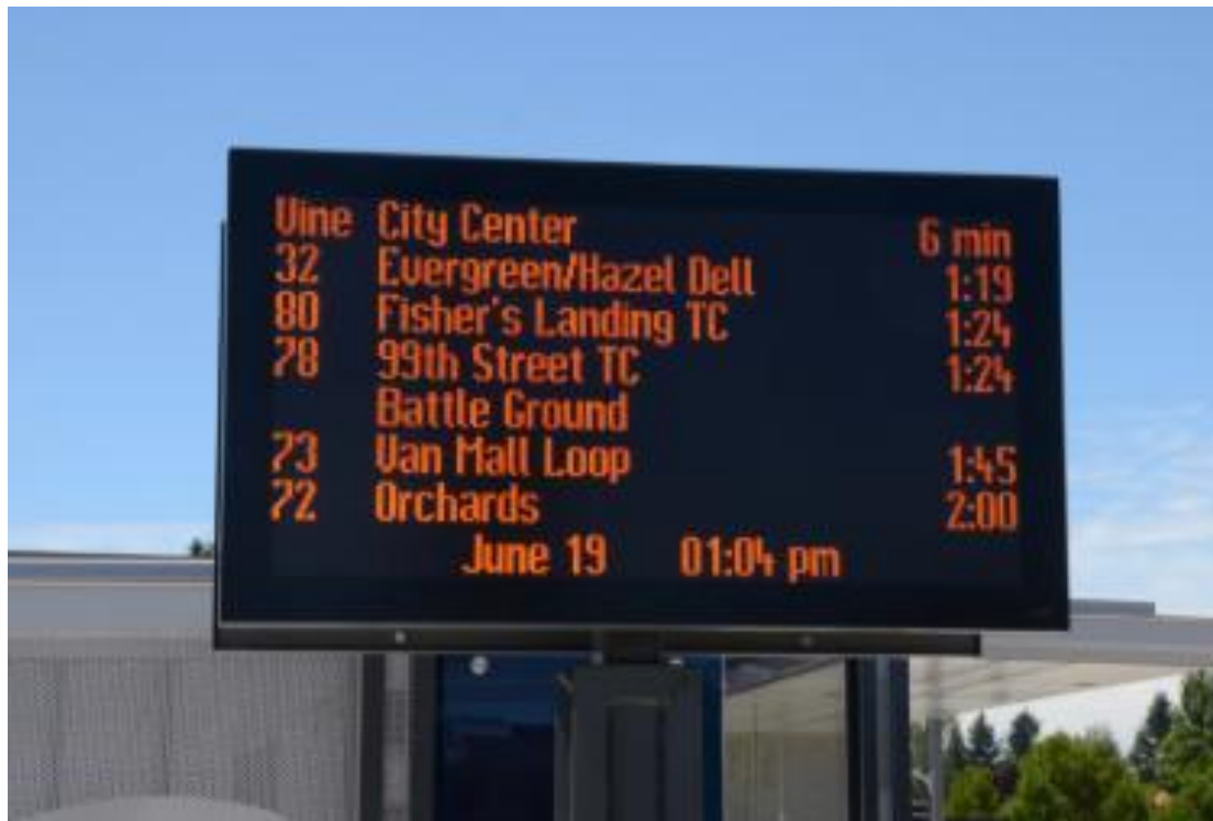
Figure 7-10: Sample "Next Bus" Real Time Information Display
