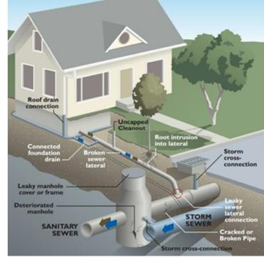
Figure 3: Typical Sources of Extraneous Flows (Note: there are no known municipal storm cross connections to the sanitary sewer system)
