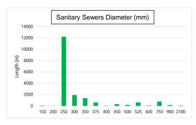
Figure 5: Sanitary Sewer Diameters
