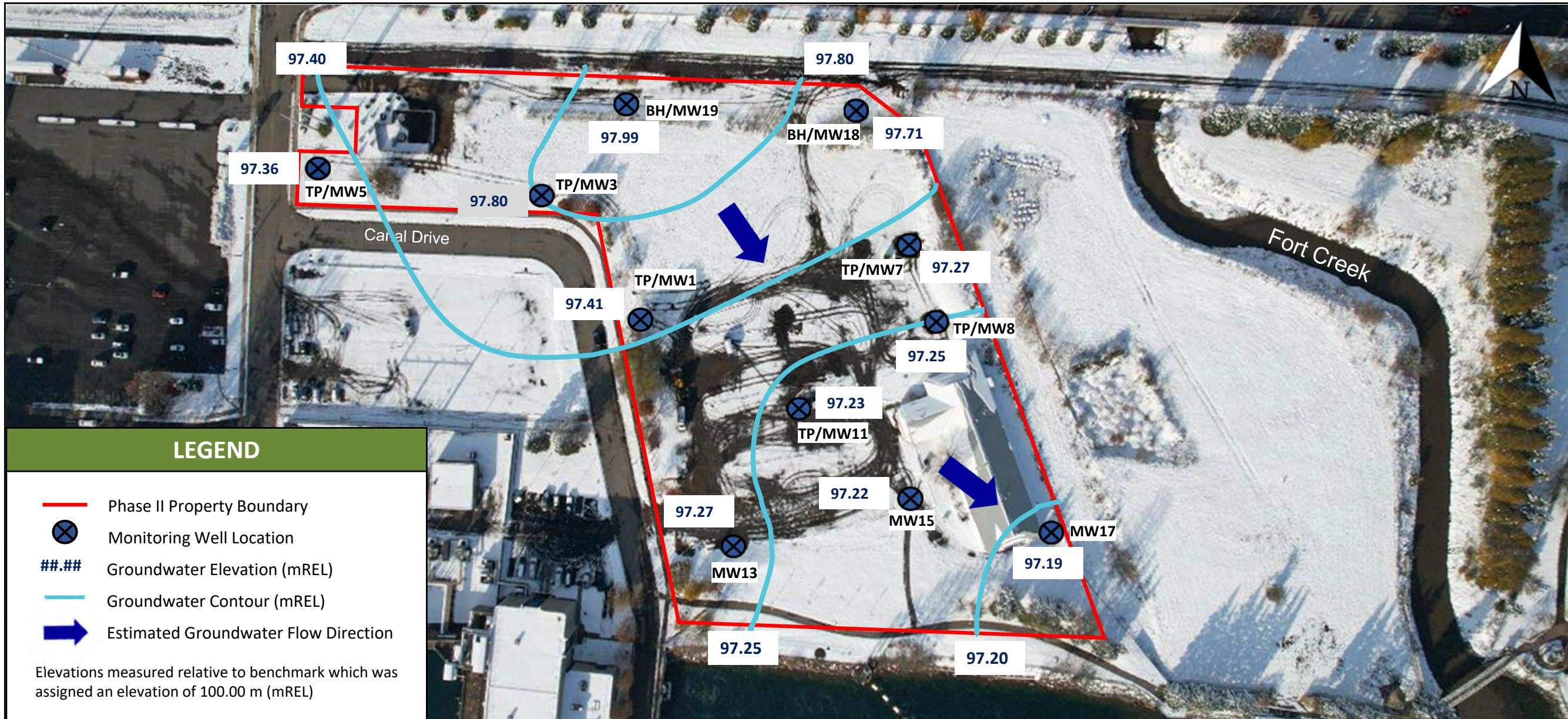
**FIGURE 6: GROUNDWATER ELEVATION CONTOUR PLAN**
