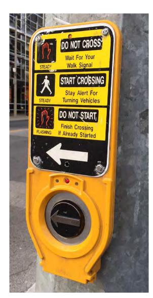
Improved accessibility with separated crossings, tactile plates, signals with audible tone and tactile buttons
