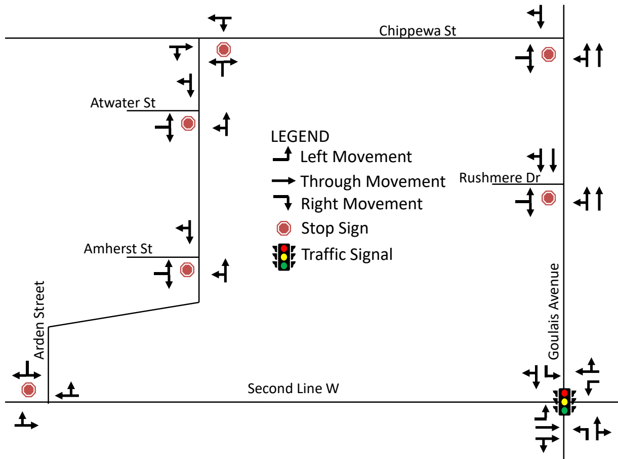
Figure 4: Existing Lane Configuration
