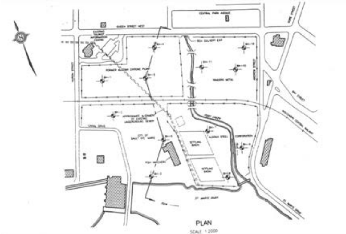
Figure 1: Borehole Location Plan.
