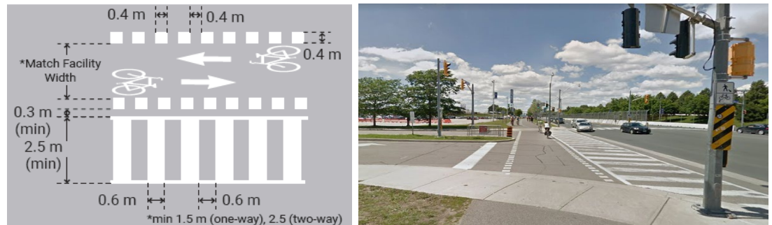
Figure 8: (From left to right) A diagram illustrating the dimensions of a Separated Crossride and a photo of the Martin Goodman Trail in Toronto where applied [Source: OTM Book 18 & Google Maps, 2021]
