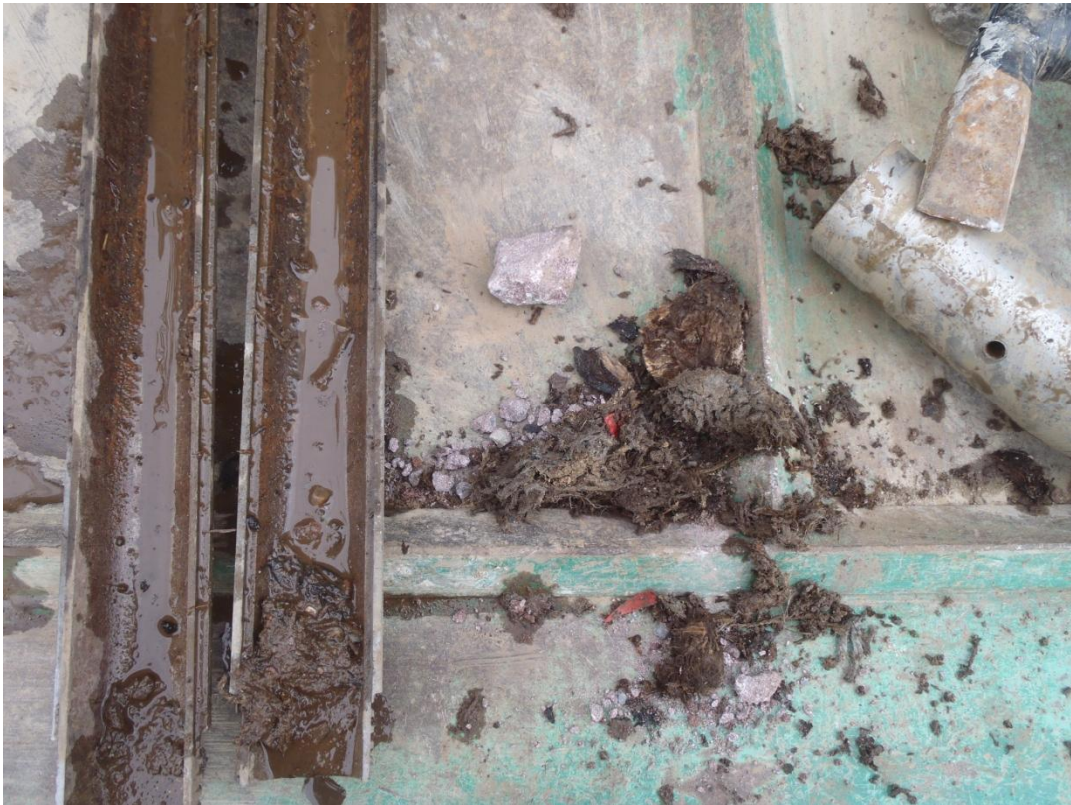
Photo 04: Waste material collected during drilling, TH13-01
