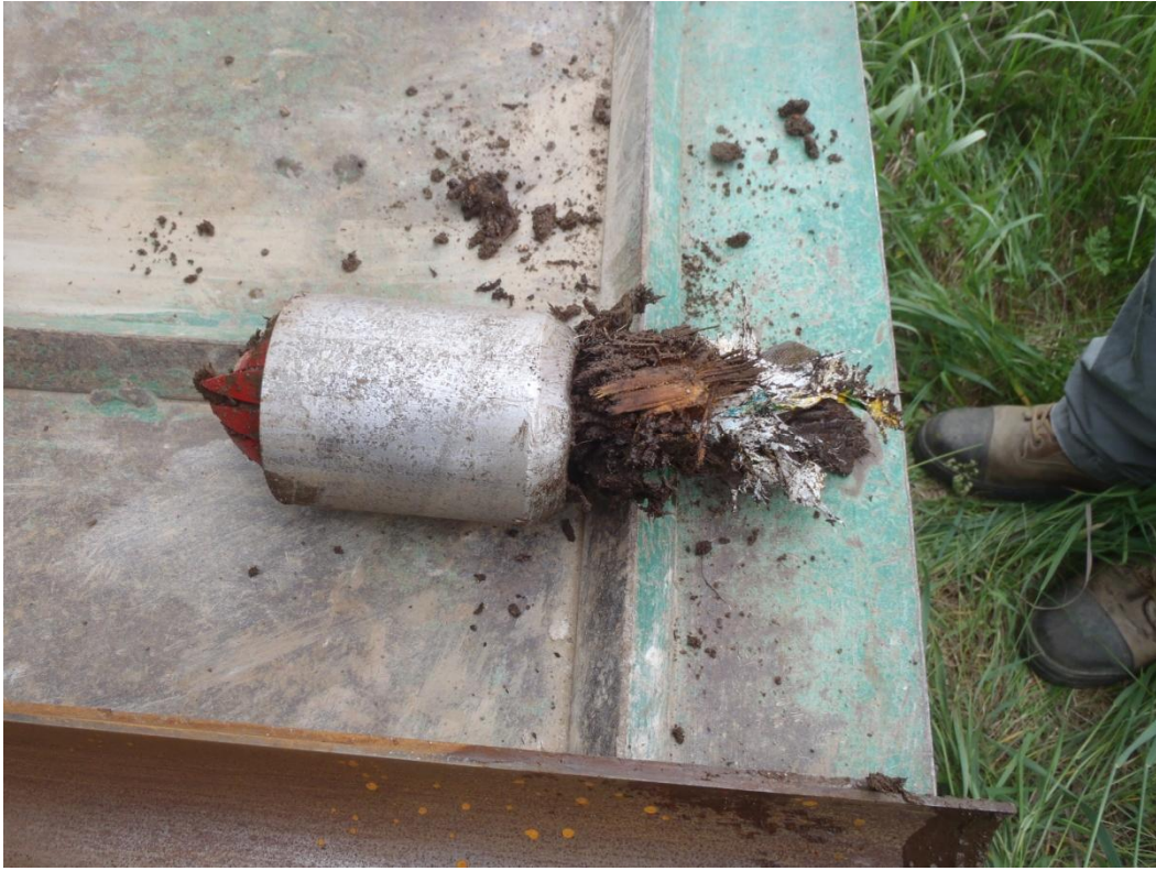
Photo 03: Waste material collected during drilling, TH13-01
