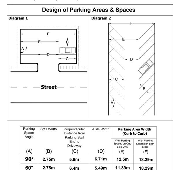
NOTE: Illustration Only. All Dimensions are minimum unless otherwise indicated. All measurements in Metric Units.
