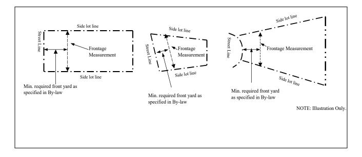
b. On a corner lot, where the side lot lines are not parallel, a tangent shall be drawn along the front lot line and the exterior side lot line extended to a point. Frontage shall be measured along a line parallel to the front lot line, between the side lot lines or projections thereof, measured from a distance equal to the required front yard of the zone in which the lot is situated.
