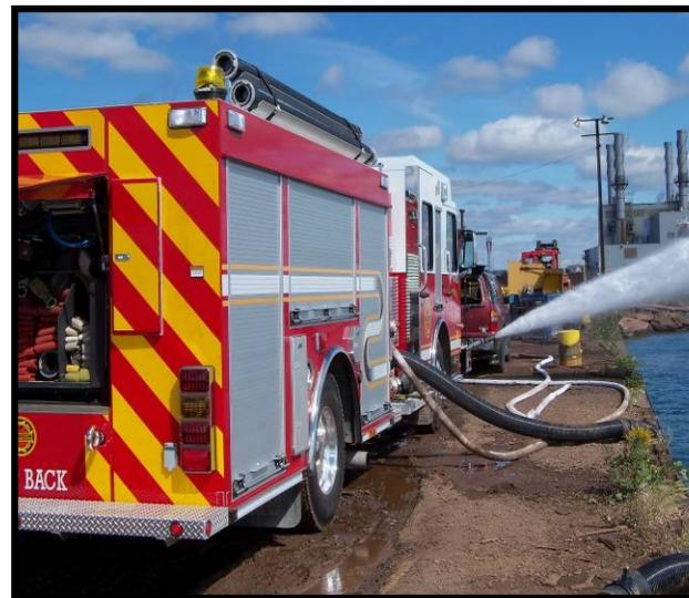
Other testing involves non-destructive testing of aerial and ground ladders as well as pump flow capacity ratings on all units with a fire pump.
