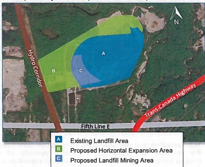
Conceptual Layout of Proposed Landfill Expansion Area
